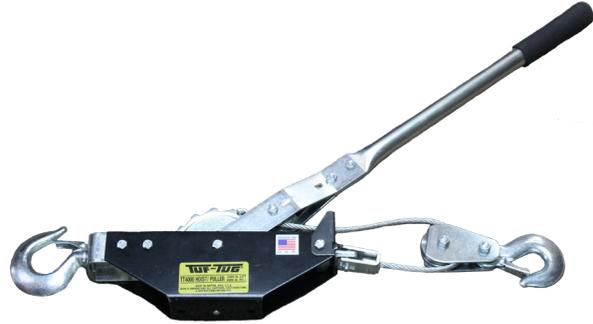
**Description** Cable Come-A-Long for use with the SafeLink Horizontal Lifeline System. Comes with 12 ft (3.66 m) of 7/32 in (5.56 mm) Aircraft cable to adjust tension in the Mobile SafeLink Horizontal Lifeline System. Come-A-Long must always be used in conjunction with the SafetyLink Adjustable Safety Strap. **See SafeLink User Manual for installation instructions.**
